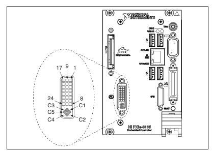
Figure 3-2. DVI Connector Location and Pinout
